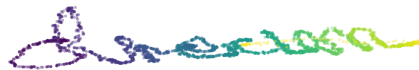
Figure 2: Reconstructed word "dream" that was recorded using horizontal and vertical (2D) EOG. Each dot represents a 2D EOG data point; the color from purple to yellow marks the time.
